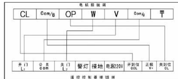
Segregated Control box and motor wiring diagram
